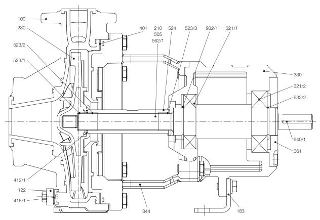
Fig.: Long life grease lubrication Mechanical seal: not shown here
